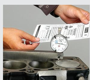
**IMPORTANT:** Compare the thickness of the previous gasket with the one that will be used (if possible, using a micrometer). When selecting a gasket, the notches that identify thickness are important (diesel engines) but also take into account that the new joint must be approximately 4% to 8% thicker than the gasket that was previously used.
