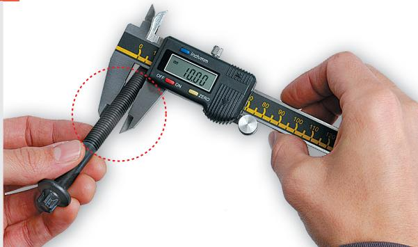
**2** Measurement of thread pitch
