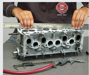
**PIECE OF ADVICE:** As a general rule, if a cylinder head of an engine that has a layer gasket is disassembled and only the upper section is being repaired (meaning that the block is not being disassembled), you should use a Metalgraf® gasket to assemble it since this will better tolerate the differences that might be in the block blueprints. When choosing a gasket, consider the variation that exists in the compression relation.
