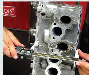
Remember that the reduction in the combustion chamber will cause temperature and pressure increases that will force the engine components. In these cases, the cylinder head gasket acts as an engine "fuse" since that is the first part to fail. If this didn't happen, serious engine damages would soon arise, such as drill holes in the piston caused by detonations (engine backfire), burnt valves, ring damages, cam misalignments, etc.
