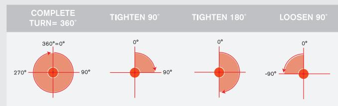
Another thing to have in mind is that grades are cumulative: if we can't turn 90° at once because there is not enough room, we can do it in stages until we reach the 90°. For example: we can have three stages of 30° since  $30^\circ + 30^\circ + 30^\circ = 90^\circ$ , or in two of 45° ( $45^\circ + 45^\circ = 90^\circ$ ):
