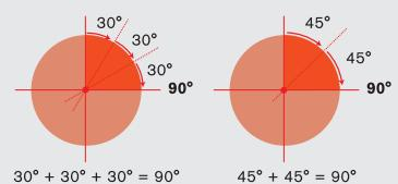
**ADVICE:** When using the angular method, the tightening must be applied all at once firm and evenly. If you stop the tightening halfway or loose the tautness that is being applied before reaching the final position, it is likely that the applied torque won't have the value specified by the manufacturer.
